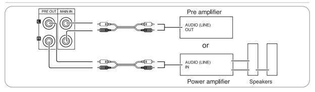
· You can connect either a pre amplifier or a power amplifier to this receiver.
